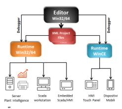
chart shows how flexible applications can be deployed.
