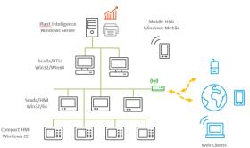
Thanks to the Movicon 11 extreme connectivity, you can communicate with any industrial device, PLC, fieldbus, instrumentation, remote I/O. All the well known producers (Siemens, Rockwell, Schneider. Omron. GE Fanuc. Saia. Web Clients Internet Access
